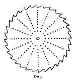
If, however, in the process of regulating the tension, you find the saw to be a trifle dishing, lay it on the anvil with the full side up, and hammer lightly over body of saw, as in Fig. 3 until you have made it perfectly flat on the log side.
