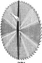
Now, put saw on the arbor, and, if for a high speed, it should sway gently from side to side in getting up to full speed. and will then run steadily and do its work properly. But if it acts as heretofore stated (that is, snaky and rattles in the guides) it needs to be more open towards the center.
