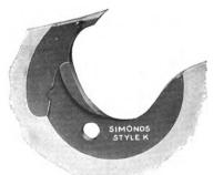
The special feature of this tooth is that a greater numbe of teeth may be carried, yet each tooth has a large open gullet. An examination of the construction of the tooth will show this large gullet room and also a swaged shank t aid in carrying off the sawdust and keeping the plate cleared. Points, shanks, and plate have a close fitting machine milled "V" and groove.
