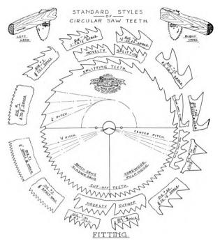
**Rules for Splitting Teeth.** The least hook that the teeth of a splitting saw should carry is tangent to a circle half the diameter of the saw: that is, the line of the face of the tooth should not pass inside a point one half the distance from the center to the rim. In most cases a little more hook than this is better; but it should never be less.
