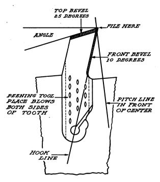
case with some slasher, trimmer, and circular gang saw rigs. The hook can be taken out and any degree of pitch in front of the center given by simply filing the point of the tooth to the desired angle. It is not necessary to file a long pitch line— $\frac{1}{16}$  to  $\frac{1}{8}$  inch is enough. This does not reduce the cutting wear of the tooth.
