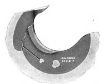
This tooth is for fine tooth saws. As many teeth can be inserted as the diameter of the saw less two; for example in a 50-inch saw 48 teeth, in a 66-inch saw 64 teeth.
