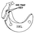
The IXL tooth, which is sold exclusively by the Simonds Company, is equipped with a key on the inner side of the point, as shown in the above diagram. This key prevents the point being forced sidewise in the shank. The three following styles may be obtained either as plain chisel teeth or as IXL teeth.
