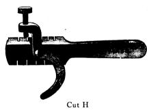
Set. Cut "H" represents a finely constructed tool for setting the points of teeth in small rip and cut-off saws. We consider it the best thing of its kind on the market. This is a combination tool having a gauge attachment for the purpose of regulating the set. It can be seen that this set is provided with setting slots which are so graduated as to give the desired depth to the set in each gauge of teeth they are intended to set.
