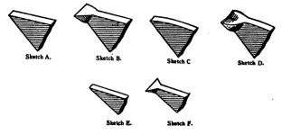
Where there is such a large amount of material in the tooth, it requires double the amount of pressure to spread it. In fact, it does not spread clear through the tooth, but simply rolls the metal over at each side of the tooth, extending quite a distance down the back of the tooth, with scarcely any in front.
