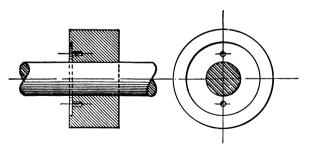
The saw should slip freely on the mandrel and close up to the fast collar. In many cases where the stem of the
