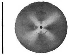
Mitre Saw. The above cut represents a circular mitre cut-off saw. These saws are ground to run without set. They are especially adapted for smooth cutting but will not cut as fast as an ordinary saw fitted with either set or swage. They should be kept perfectly round and true on the edge and filed flemming back and front of teeth.
