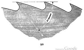
This sketch opposite is a good one to use as a guide for the proper shape of shingle saw teeth. Notice that one line is drawn straight across two teeth and one drawn following the hook of the tooth. The angle formed is 50 degrees.
