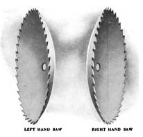
When ordering Concave Saws give circle to be dished to, or give the duameter of the old saw and the amount of drop in the old saw, accurately measured; also give the greatest diameter of the heading to be cut. State which side is to be dished or concaved, right or left hand, as the saw runs towards you
